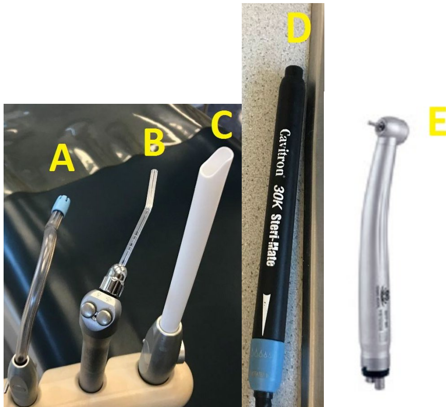
Figure 3.3 Selected Dental Instruments for Octave-band Sound Pressure Level Analysis A- small suction, B- compressed air, C- large suction, D- cavitron, E- hand pieces.
